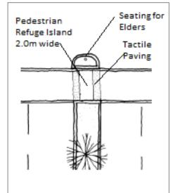
"Two type of crosswork proposed. One is Raised Crosswork, which acts as traffic calming and Other with ramp (Slope 8%) to facilitate hassle free movement for physically disabled citizens. shown in image 3 & 4, median width proposed 2.0 m, as it is proposed considering wheelchair person. As shown in 2<sup>nd</sup> image, Corporation may think to provide designer crosswork to create unique identity of Surat city"
