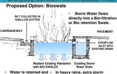
Water is retained and • In heavy rains, extra storage infiltrated in the biowater overflows into the existing S.W. Drain.
