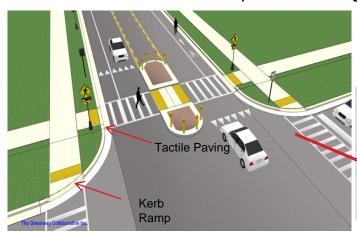
Location of Kerb Ramp must align with the Zebra Crossing location and the location of Kerb ramp on the opposite side.
